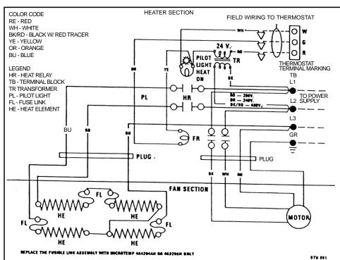
Figure 5 - Wiring Diagram
